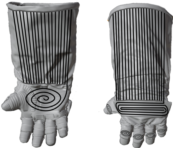
Fig. 4: Palm and back side of Artemis xEMU suit glove with AEGIS interface.
